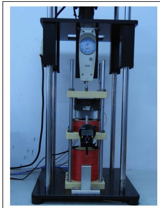
Fig. 6 T.I.M. test fixture based on ASTM-D5470
