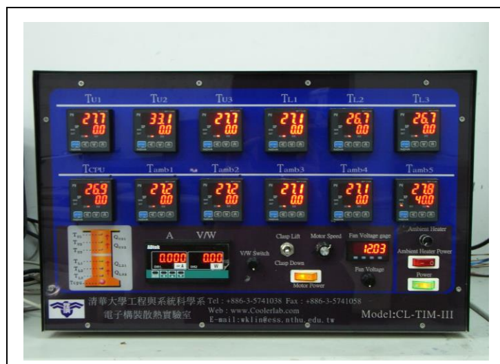
Fig. 7 Power supply for T.I.M. test Instrument based on ASTM-D5470
